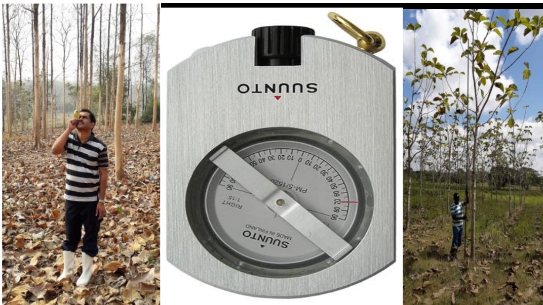
Figure 2.3. Total Tree height was measured by hypsometer and a pole, used instrument of sununto meter is shown in above.
